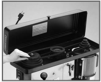
Figure 24. Adjusting belt to desired speed.
